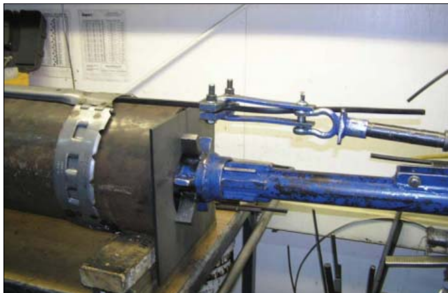
A pull and push test verified the forces needed to move the line in the 10 3 / 4 -in. clamp and move the clamp against the pipe (Fig. 1).
